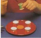
6) Place the hole in the center of the turbine over the pin
