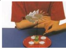
7) **TO BE DONE BY MENTOR:** Light the candles. The hot air from the candles should spin the turbine.
