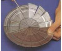
Angle the blades by holding the inner tip and twisting the outer edges 20 to 30 degrees. The center of the inner tip should be flat, in line with the center of the disk.
